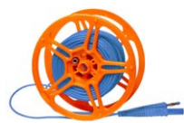
Test lead for earth resistance measurement 25 m
